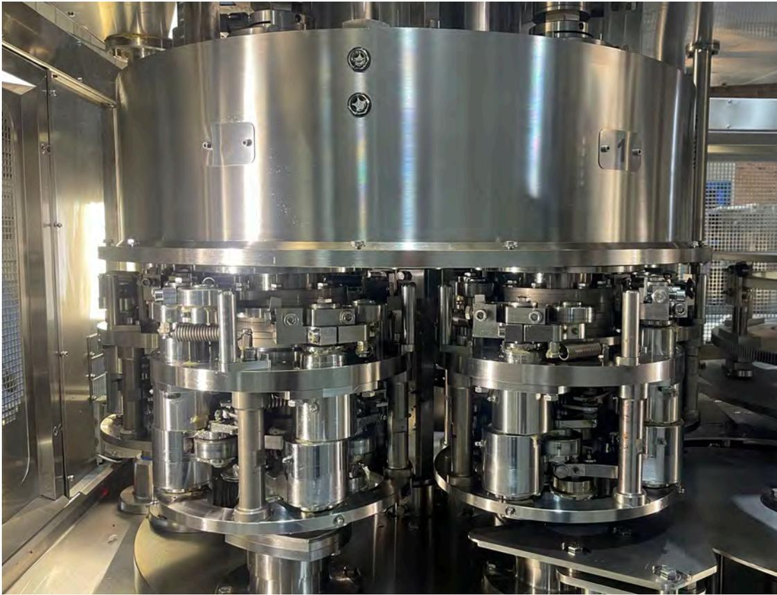
**Left** An MCG F-640 seamer featuring the new patented seaming heads, enabling lower gauge cans to be packed
