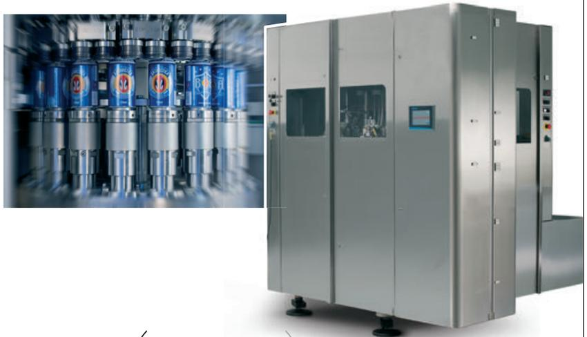
MCG's F640 irregular can seamer has recently been further improved by the re-design of the piston clinching station to further reduce spillage. By stepping down from 12 pistons to nine, and re-engineering the station to use a cam and eliminating the use of springs, spillage is reduced to a minimum and less maintenance is required.
