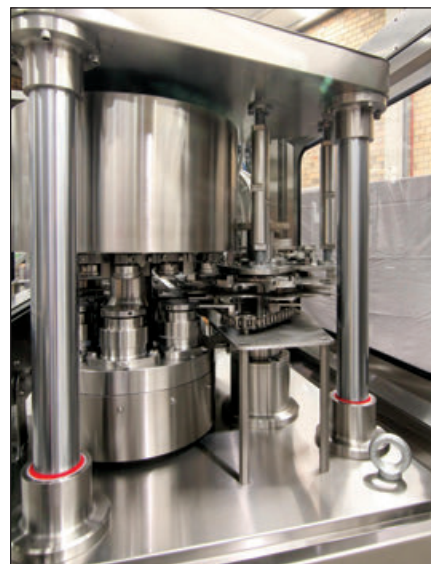
Mexican food processor Productos Carey uses Angelus seamers and parts from American Holt; and right, MCG's R645 round can seamer
