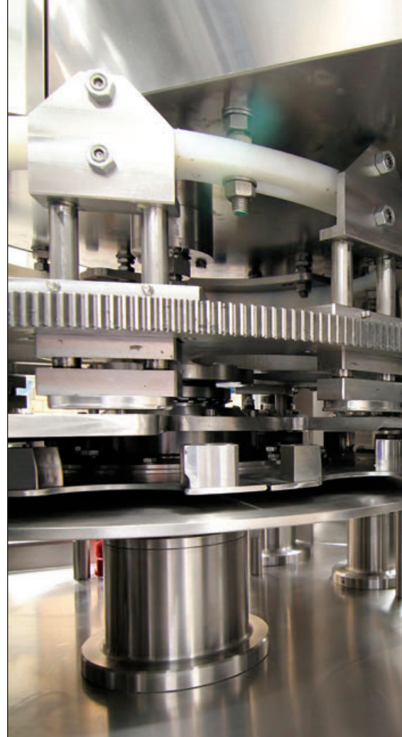
MCG's F-113 seamer with automatic height support columns, and the company's trademark full stainless steel finish
